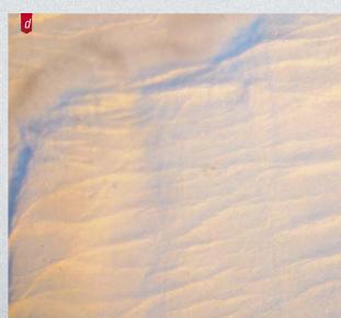
The inner surface of synthetic vascular prostheses used in current surgical practice is very rough, hairy, and unable to maintain the development of a normal cell layer unlike the prostheses produced by electrospinning:
