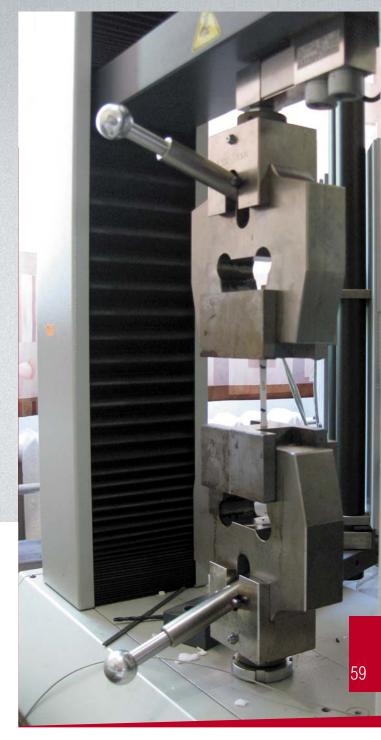
The material produced by electrospinning has been tested for mechanical properties in a Zwick/Roell Z100 machine at the joint access center for mechanics with the Lavrentiev Institute of Hydrodynamics, Siberian Branch, Russian Academy of Sciences (Novosibirsk). Photo by the courtesy of A. Lebedeva
