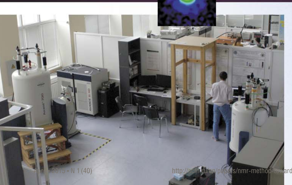
Left: New powerful NMR spectrometers at the International Tomography Center (Novosibirsk); one of the spectrometers (with a working frequency of 700 MHz) was purchased using the mega-grant funding Top left: An MR image of a phantom filled with hyperpolarized propane and a sphere filled with water
