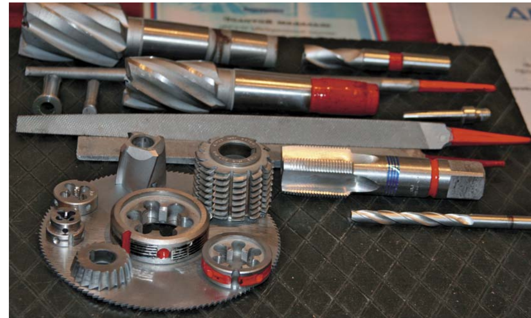
When nanodiamond coating is applied onto the cutting edges of mechanical tools, their service life becomes much longer
