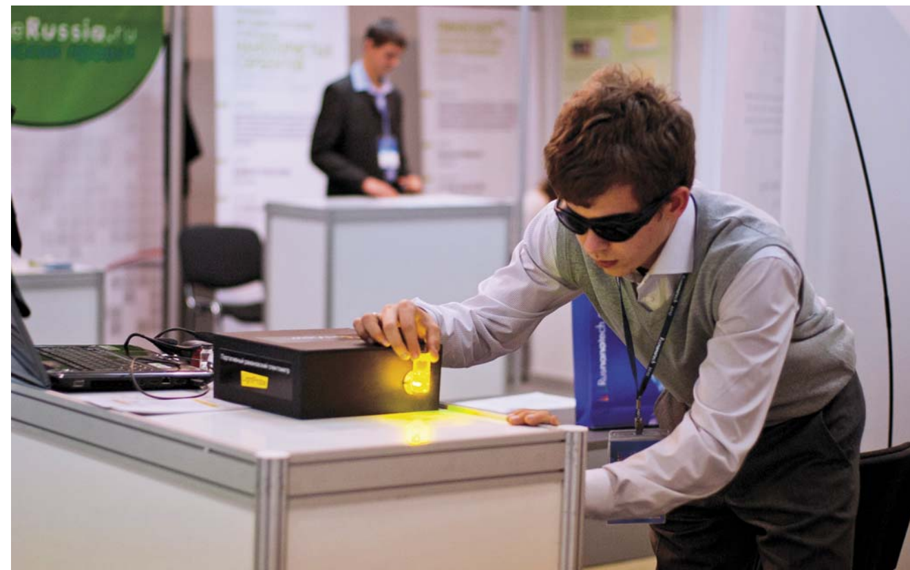
Using the new optical analyzer, one can determine the chemical composition of the substance rapidly and accurately, even through bag walls. In the photograph , D. A. Gavrilov, one of the analyzer developers, is demonstrating its capabilities at the RusNanoTekh-2010 exhibition (Moscow)
