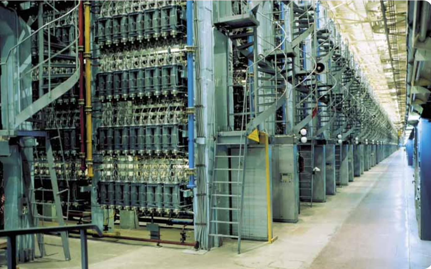
Separation of ^{235}\text{U} and ^{238}\text{U} isotopes in centrifuges. Gas flows of enriched and depleted uranium hexafluoride are directed by ducts around the cascade of centrifuges which work as a united system having an efficiency close to 100%
