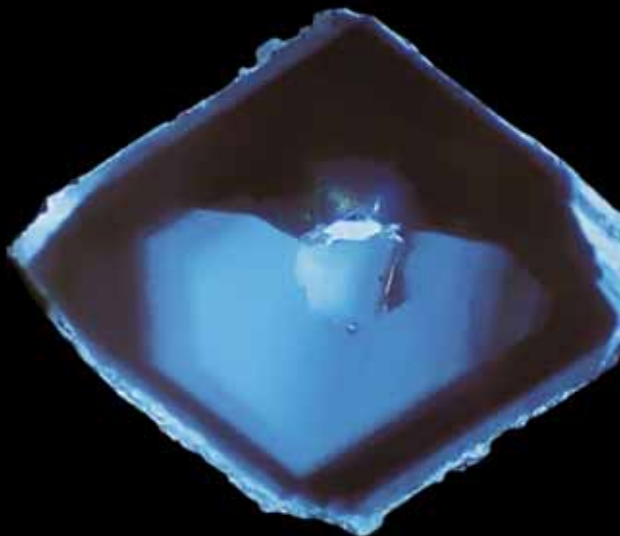
A pure diamond that has had “a hard life”. This snapshot shows the diamond’s “life story”: you can see that the conditions were changing (the areas differ by intensity and color of luminescence)
