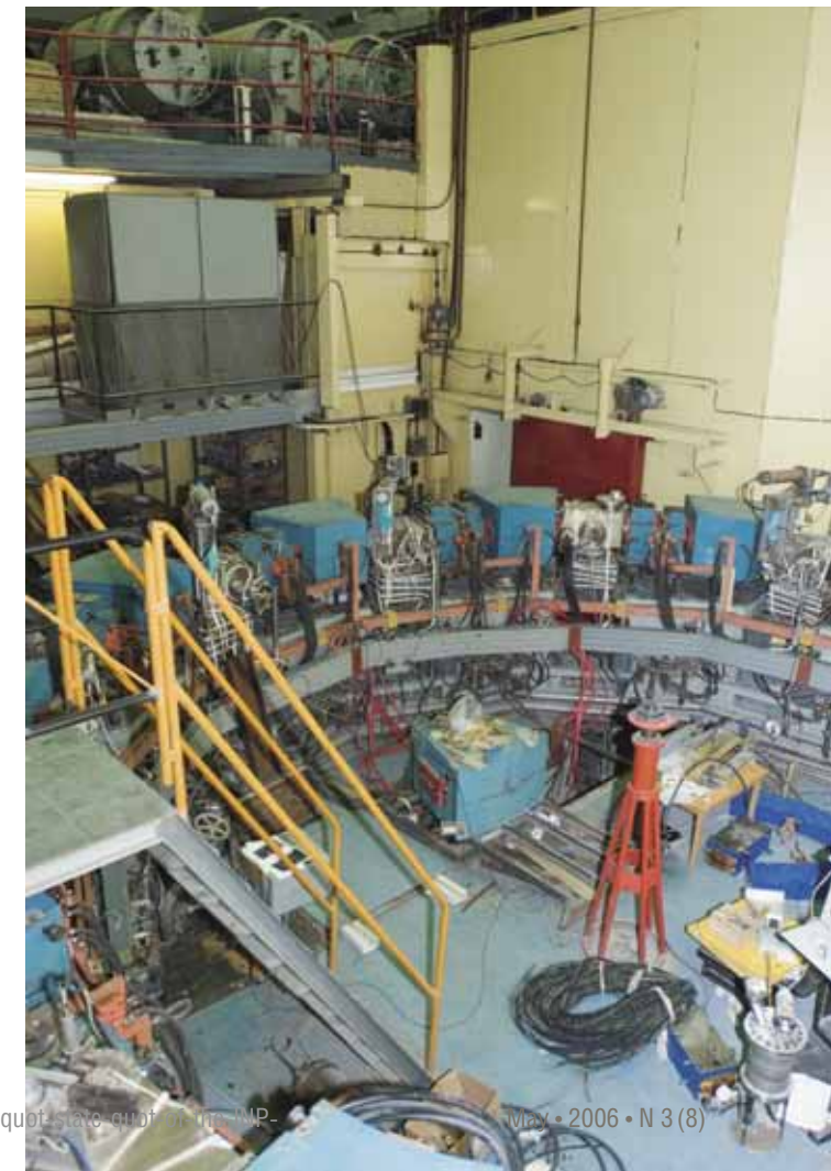
VEPP-2M complex operated within the range of energies from 0.4 to 1.4 GeV. The maximum luminosity reached was 5 \times 10^{30} \text{ cm}^{-2} \times \text{sec}^{-1} with an energy of 510 MeV
