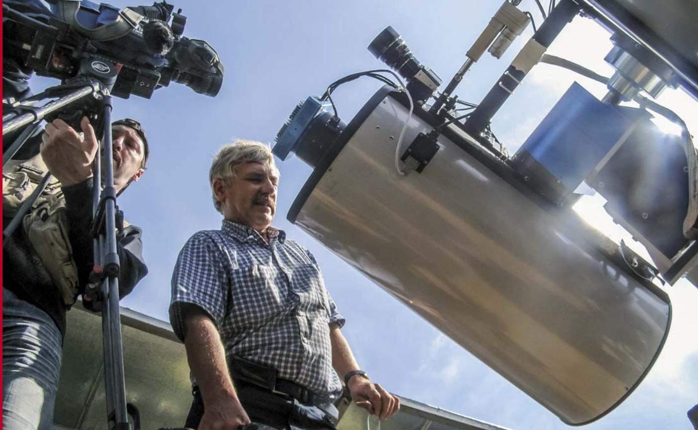
This twinned MASTER-2 telescope installed on the astrophysical test site of Irkutsk State University in the Tunkinskaya Valley is one of the first completely automated systems for monitoring celestial objects in Russia.
