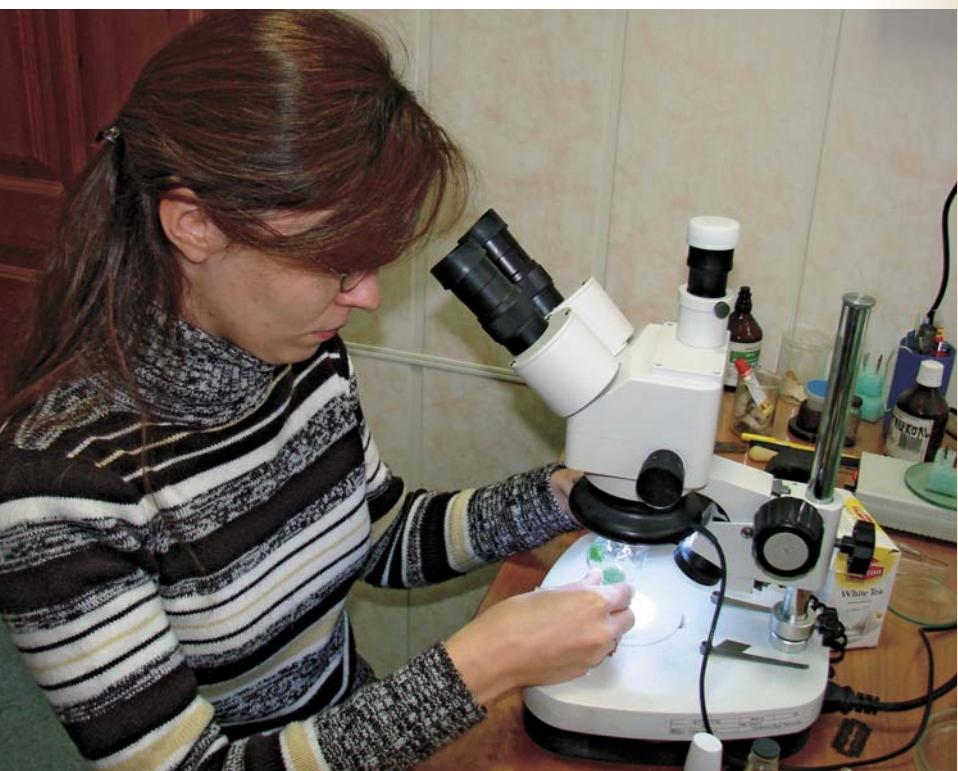
The first task is to select among many crystals the one most suitable for analysis. Then, it should be attached, for example, to a 20 µm thick nylon loop connected, through a special sample holder, with a fine regulation screw for micro-scale positioning
