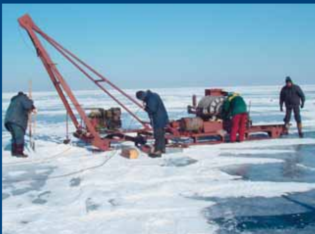
Shallow gravity sediment cores were retrieved from the ice above the venting sites during the winter trip of 2000 organized by the Limnological Institute in Irkutsk. Photo by N. G. Granin
