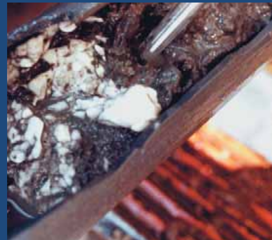
Gas hydrates recovered by gravity coring appear as white opaque inclusions of two types: massive lumps enclosing thin fissures filled with sediment, and numerous inclusions in the sediments up to 2 cm in size, isometric and plate-like in shape. According to gas chromatography data, methane is the dominant component of the hydrated gas (up to 99 % of total hydrocarbons).
