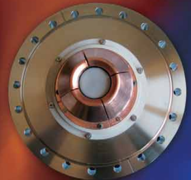
Another idea extending the capabilities of electron cooling is to divide the ring controlling the beam profile into four sectors. This idea was implemented in the novel cooler recently made for Germany
