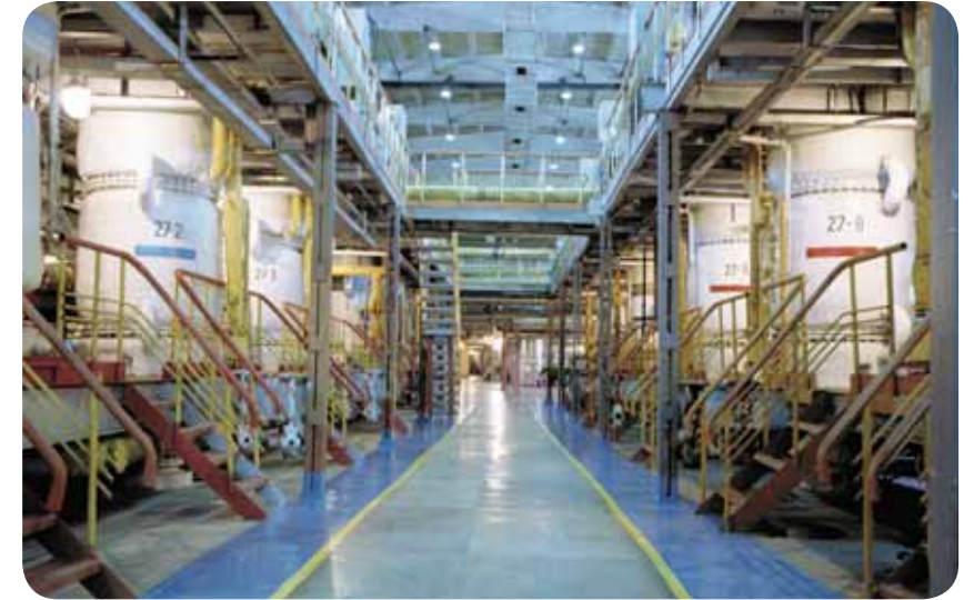
Desublimators serving to crystallize gaseous uranium hexafluoride
