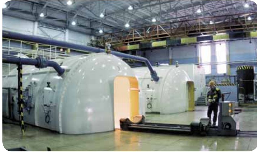
Production unit for pouring and packing finished products. Special-purpose machines called "shuttles" fill containers with uranium hexafluoride in its liquid aggregate state. The product is then crystallized and packed for transportation
