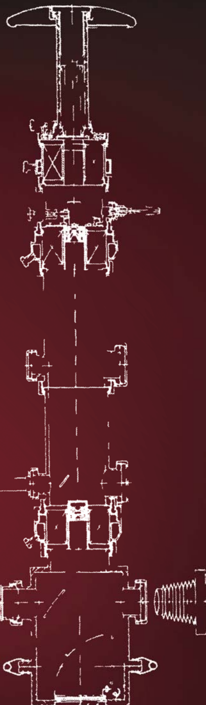
Author's sketch of the first two-stage electron microscope (the microscope column cross-section was redrawn in 1976)
