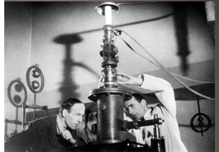
Knoll and Ruska with their first electron microscope. Berlin, 1944. Credit: Ernst Ruska Archive, Berlin (Germany)
