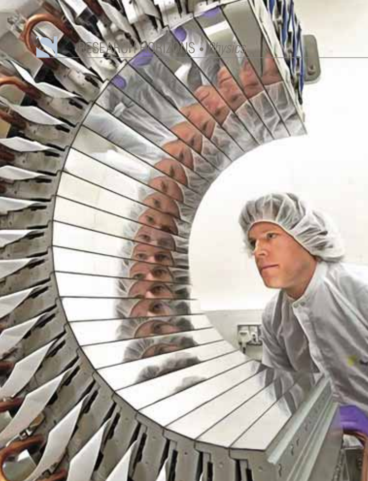
The structure of native proteins and nucleic acids is determined using a vacuum X-ray diffractometer. These studies must be conducted in vacuo because soft X-rays are strongly scattered in air. Courtesy of Diamond Light Source
