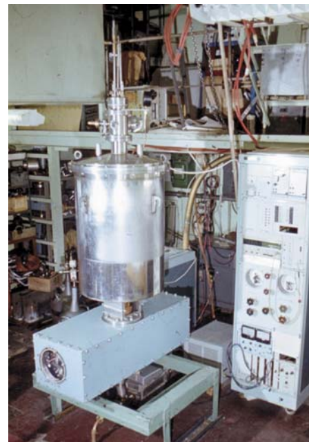
The first superconducting wiggler in the world, which was fabricated by BINP SB RAS in 1979 ( on the right ), consists of two rows of short superconducting magnets with alternating polarity. The magnets generate a variable-sign dependence of the magnetic induction of the field on the longitudinal coordinate, which is close to a sinusoidal curve. In such a field, the charged particles move along a serpentine curve in the space between the magnets, the curve resembling a snake's path. The photograph was taken by the author
