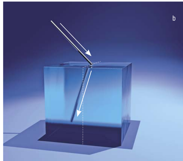
Schematic illustration of light refraction in the systems 'air – conventional positive-index material' (a); and 'air – negative-index metamaterial' (b)
